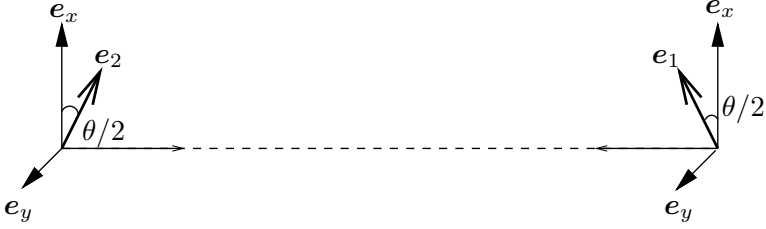
Fig. 6. The schematic of a \text{lin}\theta\text{lin} configuration. Two linearly polarized light beams travel along the z -axis in opposite directions, with the angle between the polarizations \theta .
